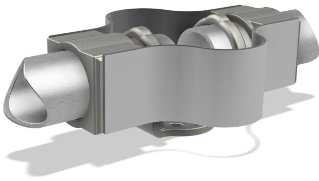
The "WRX" with suffix "W" is an all welded aluminum expansion connector with welded laminated shunts. Shunt material is #1100-0 aluminum alloy with each lamination .020" thick for maximum flexibility. Cast parts are #356, heat treated to T6 temper. Lamination is designed for maximum of 2,000 ampere service at 30°C rise. For higher ampere rating, specify at time of order.
