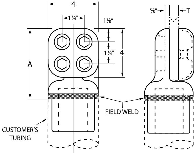
Types "WL" and "WL-CF" welding terminal lugs have extra heavy castings, recessed bolt heads in the pad and are supplied with bolt shields to protect against corona. Customer to specify "T" dimension so correct length of hardware can be furnished. Type "WL" is a side formed lug as shown in Figure. Type "WL-CF" has the terminal pad on the same line as the centerline of the tubing. 4" x 4" pad. For up through 550 kV. Welding terminal lugs are also available for 15°, 30° 45°. and 90°.
