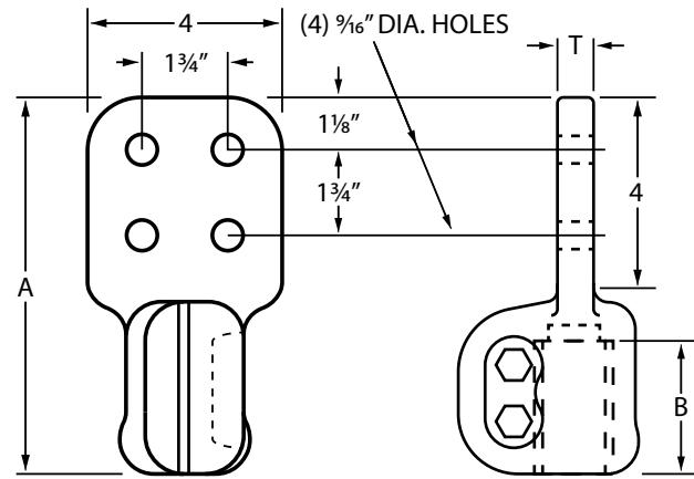
The "SBES" stud connector is an aluminum bodied unit designed for making a flat pad connection to an aluminum equipment stud. Connectors will carry the full rated current of pad or stud, whichever is smaller. For up through 550 kV using bolt shields.
