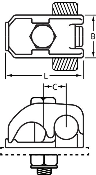
Grounding connector for clamping a single grounding conductor to a flat surface such as a steel structure or equipment housing. Cast of high strength copper alloy, body of fitting will accommodate a wide range of cable sizes. Bolts, nuts, and lock washers are of hot galvanized steel to resist corrosion. Bolts of sufficient length to grip 1/4 inch thick bar are standard. Bolts for greater thickness can be supplied when specified.
