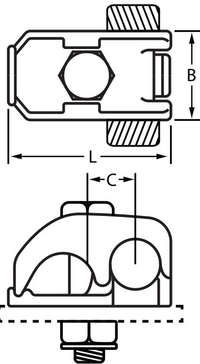
Type "GFS" connector is designed for clamping a single grounding cable to a flat surface such as a steel structure or equipment housing. Bolts supplied are of sufficient length to grip 1/4" thick bar. Specify at time of order if thicker bar.
