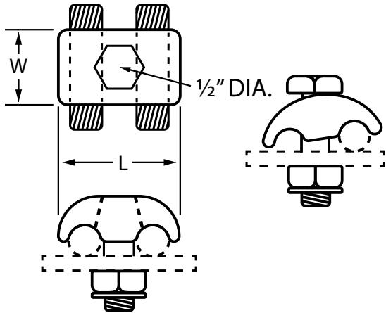
GFH ground clamps are an economical means for clamping a single or two ground conductors of unequal size to a flat surface. Bolts are of sufficient length to grip 4 inch bar. Longer bolts can be supplied.
