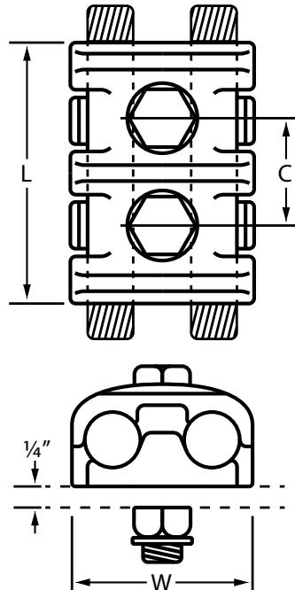
Types GFD is a two conductor grounding clamp that is simple in construction, yet designed to permit a single fitting to be used for a wide range of cable sizes. Body is cast of a high strength copper alloy, and is equipped with silicon bronze bolts, nuts and lock washers. Bolts of sufficient length to grip 1/4 inch thick flat bar are provided unless otherwise specified.
