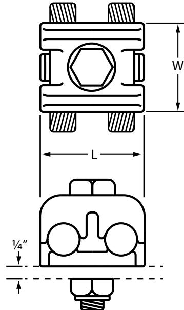
Types AFD is a two conductor grounding clamp that is simple in construction, yet designed to permit a single fitting to be used for a wide range of cable sizes. Body is cast of a high strength copper alloy, and is equipped with silicon bronze bolts, nuts and lock washers. Bolts of sufficient length to grip 1/4 inch thick flat bar are provided unless otherwise specified.
